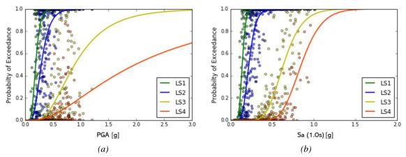
Figure 5. Fragility curves for RC MRF LR C typology with different IM: (a) PGA and (b) Sa at 1.0 sec (best fit) [Slight (LS1), Moderate (LS2), Extensive (LS3) and Collapse (LS4)].
