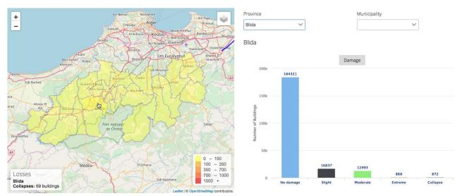
Figure 9. Damage distribution map (left) and number of buildings in different damage states.
