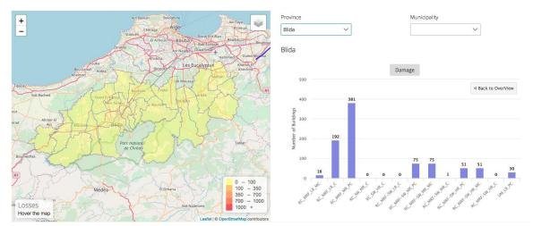
Figure 10. Number of buildings per building class associated to the collapse damage state.
